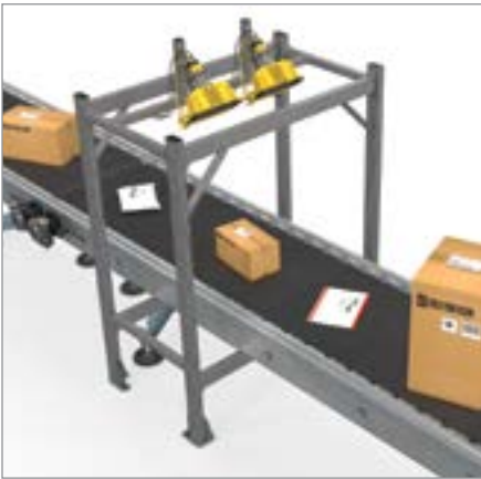
Single-, multi-, and full coverage scan tunnel options are available to help increase throughput in logistics applications. Multi-Reader Sync technology synchronizes several readers for increased field of view and multi-side scanning at high speeds.
